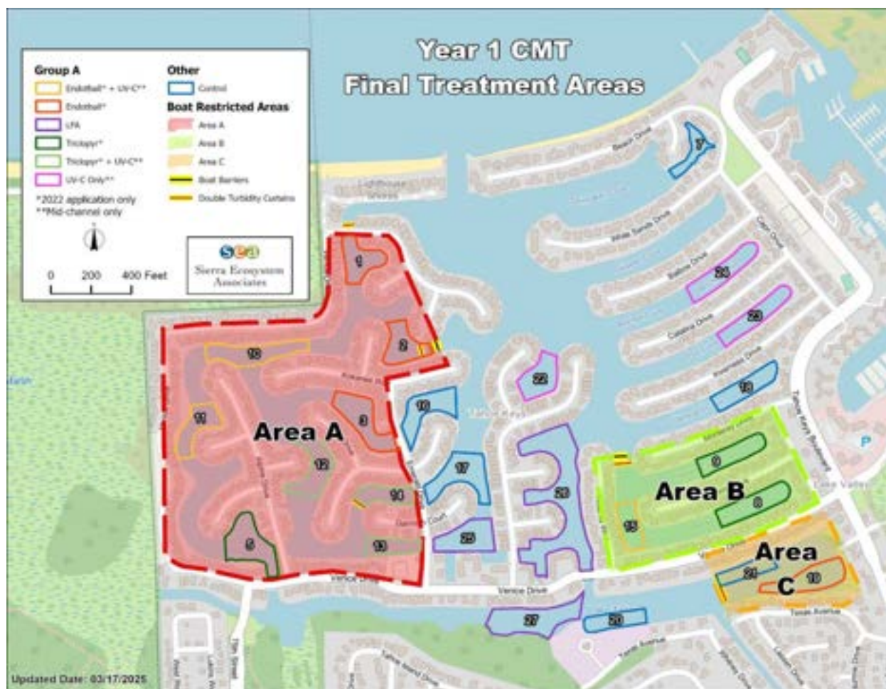
Figure 3-4. Boating restricted areas (A, B, C) during deployment of turbidity curtains. Note: At Sites 1, 3, 13, and 14, culvert plugs were installed to prevent water movement in or out of the Sites into untreated areas or toward Lake Tahoe.
